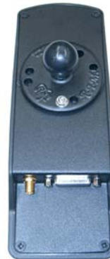
Attach Ram-Mount base to SatDOCK
